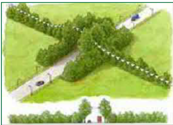
Illustration 1 Example of a hop-over which creates a flight path at a safe height above the road taken from Limpens et al. (2005)
